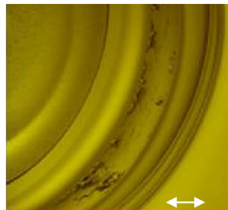
Fig. 35 Severe flaking from the cathode shielding after 23 kWh sputtering for one of the target material. Arrow = 20 mm
