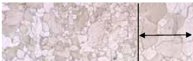
Fig. 18 Grain size difference for a surface rolled sputter target (sputtering surface on right hand side above), arrow = 200 \mu\text{m}
